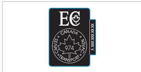
Plate confirming national emissions gas guideline values and safety requirements for motor vehicles (example: Canada, complete vehicles)
